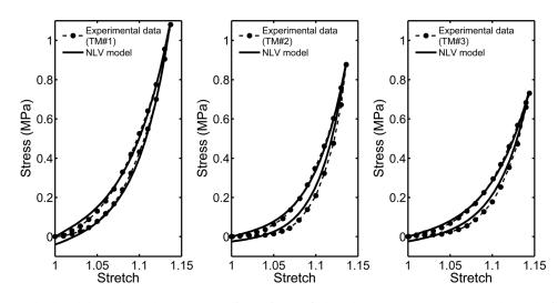
FIG. 4. Experimental data for three individual TM specimens reported by Cheng *et al.* [2007, Figs. 4(a)-4(c)] compared with simulated results from NLV model.
