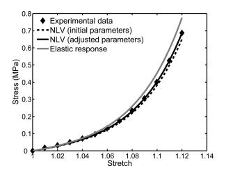
FIG. 2. Stress-stretch relationship for the mean experimental data of Cheng *et al.* (2007, Fig. 6) and for the NLV model with initial parameter values, with adjusted parameters, and with adjusted parameters but no relaxation (i.e., elastic response).
