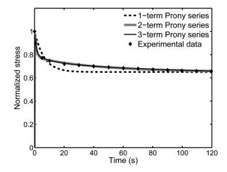
FIG. 3. Experimental data (Cheng *et al.*, 2007, Fig. 8) and comparison with simulated relaxation tests with one-term, two-term, and three-term Prony series.
