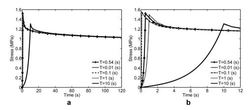
FIG. 5. Effect of loading time on simulated relaxation response of TM strips. (a) Full duration of measurements (120 s), showing lack of long-term differences. (b) Expanded view of first 12 s of response, emphasizing the short-term differences.
